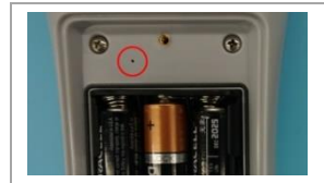
Figure 7: Alignment Access Hole Location
